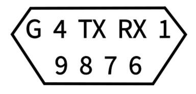
TX: transmit line; RX: receive line; G: reference potential
