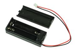
This tough battery case is built for 2x AAA batteries. It has an on/off switch and a cover. The JST connector makes this battery compartment ideal for use with the micro:bit.
