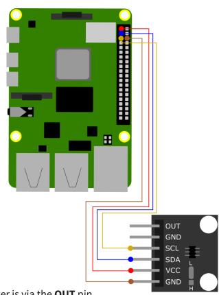
The analog output of the converter is via the **OUT** pin.
