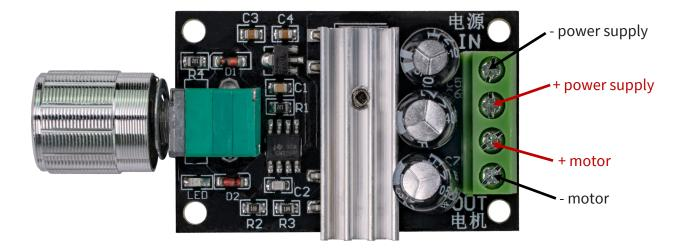
By turning the potentiometer, the speed of the motor is adjusted by  $\ensuremath{\mathsf{PWM}}.$
