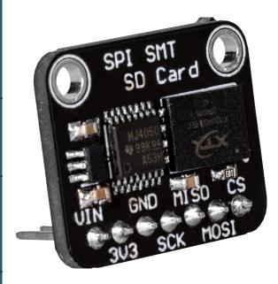
This flash memory allows you to store and read data externally via the SPI interface of your microcontroller.
