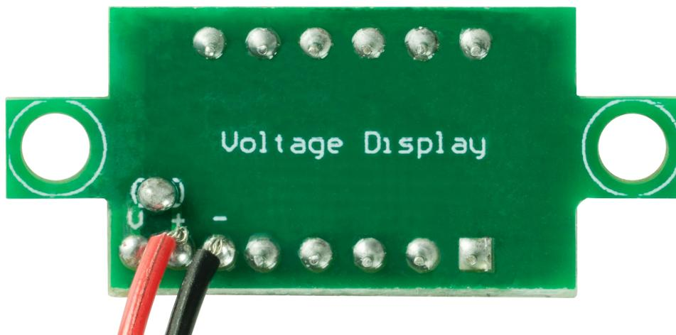
You can also measure voltages below 3 V with this voltmeter, but for this you have to supply power to the display regardless of the measuring voltage. This requires soldering, because you have to remove a solder bridge on the back of the unit and solder more wires to the board.
