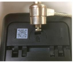
need to purchase the safety lock by themselves. Wrap one end of the safety lock around a hard-to-move object, insert the other end into the safety lock hole, turn the key clockwise to lock the instrument, and then pull out the key. In this way, the most basic anti-theft requirements can be achieved.
