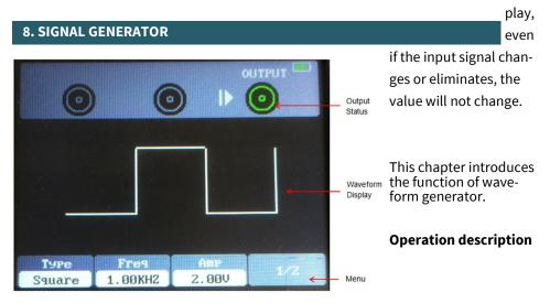
Press the power button to turn on, and then press the "AWG" button to enter the waveform generator function interface.
