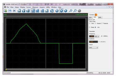
5. Draw any waves with the mouse in the waveform area.
