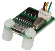
First of all, attach the spacers at the module with two nuts.
