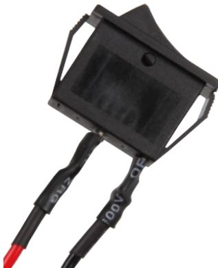
To prevent a short, you should isolate the contacts with shrinking tubes.
