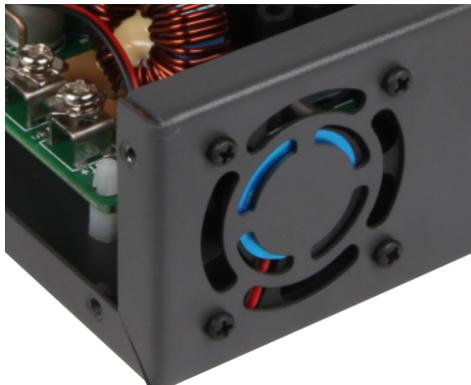
After the cables are connected and the fan is mounted, you can install the small board with two nuts at the case.
