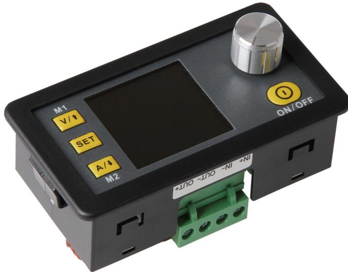
The input voltage and the output voltage of the case must be plugged in to the intended 4-pole PCB plug.
