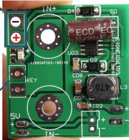
Now you can solder the switch. Have in mind that the cables must go later on through the case or attach the switch beforehand. The ends of the cables at the switch have to get soldered at the pads “KEY“. Solder the red cable on to the rectangle pad and the black one on to the round pad.
