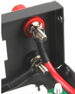
The end of the cable from the output voltage must be connected with the ports in the front.
