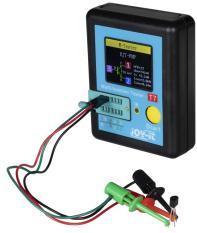
This LCR meter offers a wide range of functions at a low price. The LCR meter can measure capacitance, resistance, and inductance among other things. In addition, it can automatically recognize components, for example, it can distinguish between different types of transistors, such as NPN or PNP transistors. The device is particularly easy to operate, as all measurements are started at the touch of a single button.
