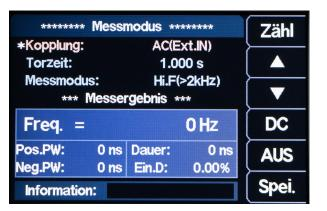
Press **MEAS** to enter the measuring mode menu and press the **CNTR.** or **MEAS.** menu button to switch between the counting and measuring functions.
