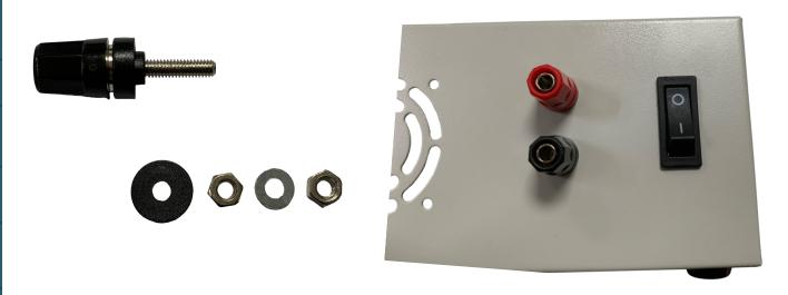
3. You can screw the black cable on the black bush and the red cable with the blade receptacle on the red bush. Therefore, you have to note that the cable lug is screwed before the washer and the other nut.
