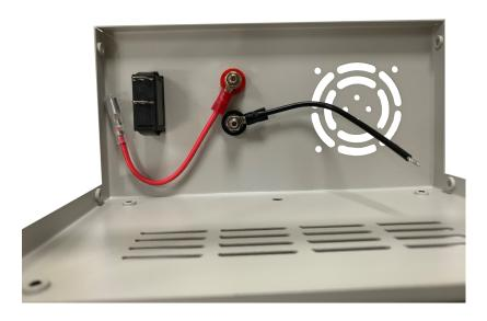
4. The cable must be now mounted with the blade receptacles on the switch. Therefore, you need to note that the cable from the bush is mounted on the position 0 and the other on position 1. Afterwards, insert the RD6006 into the case. You can affix the last loose cable ends on the module itself namely the current input terminal. Therefore, it is to note that the red cable must be screwed into the + and the black one into the -.
