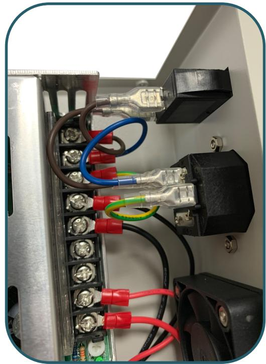
7. Now, connect the black cables of the fan controller and the RD6006 power supply unit to the V- terminals and the red cables to the V+ terminals.
