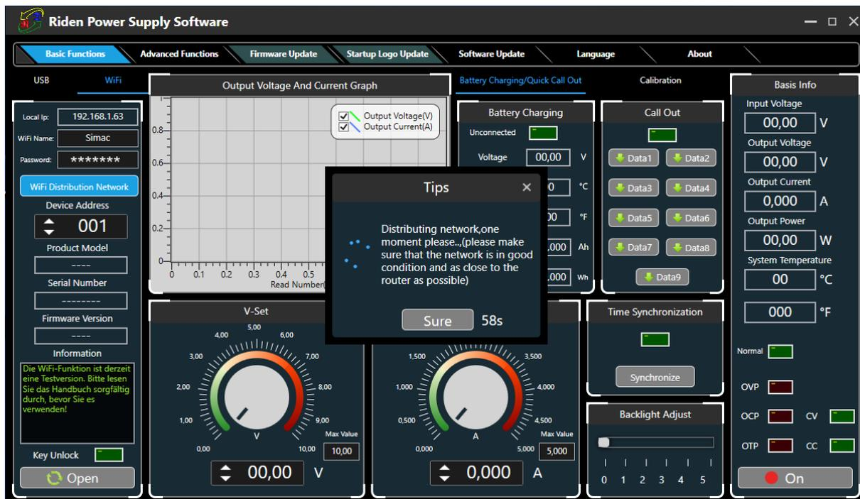
You can then connect your power supply unit to the PC software by clicking on Open in the lower left corner.
