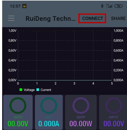
Now you can operate the power supply with your smartphone. Please note, however, that the power supply cannot be adjusted manually as long as your smartphone is connected.
