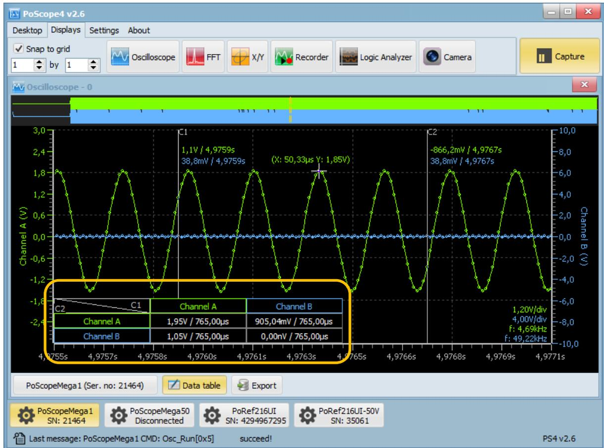
**Hint:** If you click with left mouse button in the data table you can toggle between time calculation between two cursors and frequency calculation.
