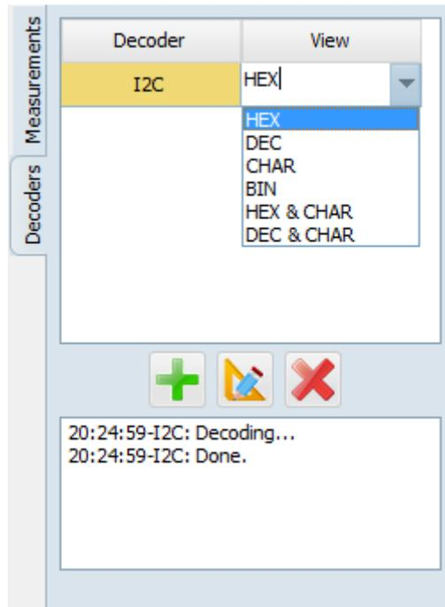
Under the View, you can select how you want the decoded data to be shown. HEX, DEC, CHAR, BIN, HEX & CHAR, DEC & CHAR are available. Measurements can be shown in the side panel or as a hint when you hover the mouse cursor over the I2C data.
