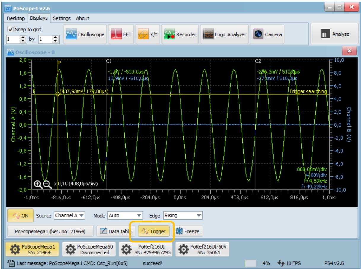
Some signals change very fast. To catch the desired event, you can use **triggering**. **Trigger** is a standard oscilloscope function that allows you to catch the live signal at some particular point so you can closely analyze it. Just choose the correct channel, select Mode (automatic loops or a single trigger) and particular edge of the trigger (signal rising / falling / any).
