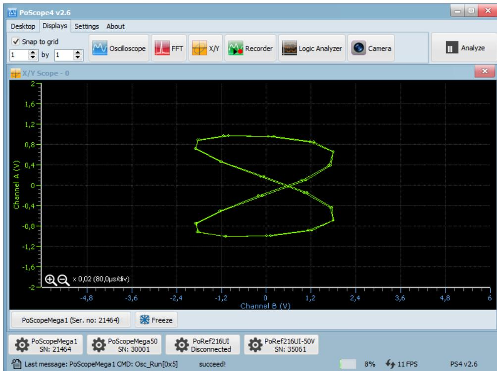
*Lissajous curves figure infinite at frequency ratio 1:2*
