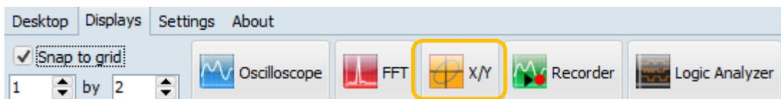
You might come across this window. In order to track phase differences, both of the channels have to be active. You have to turn on the signal on channel B on the Mega1 device control GUI.
