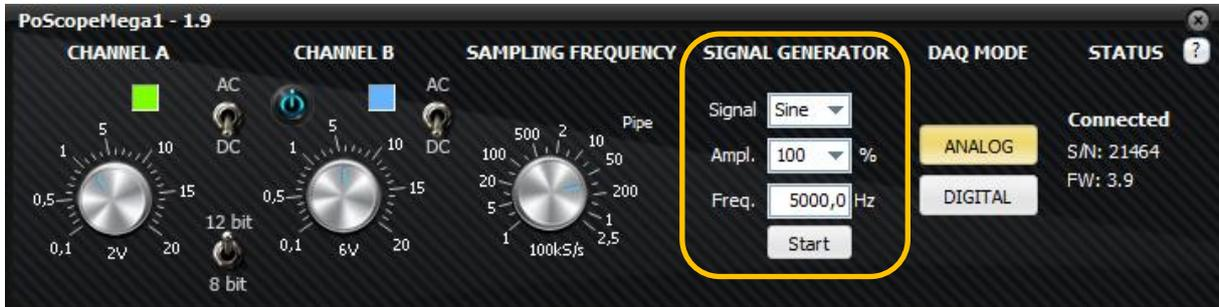
The waveforms on the oscilloscope display will change according to the shape of selected signal on the analog generator part of the Mega1 controls.
