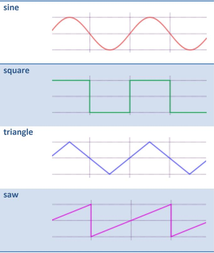
To show you the basic use of function generator, we connected two probes to the PoScope Mega1+, first one to the function generator output and the second one to oscilloscope channel A. We connected the signal and the ground connections of the two probes and ran the function generator at 5 kHz.
