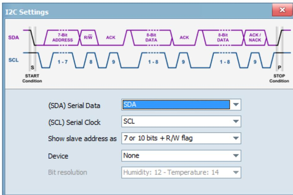
If you name your pins as I2C standard names (SCL, SDA) the decoder settings window will automatically recognize lines and use them for decoding otherwise you have to manually select pins for data sources.
