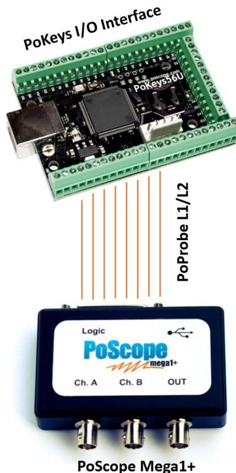
*Logic analyzer measurements on PoKeys I/O controller*
