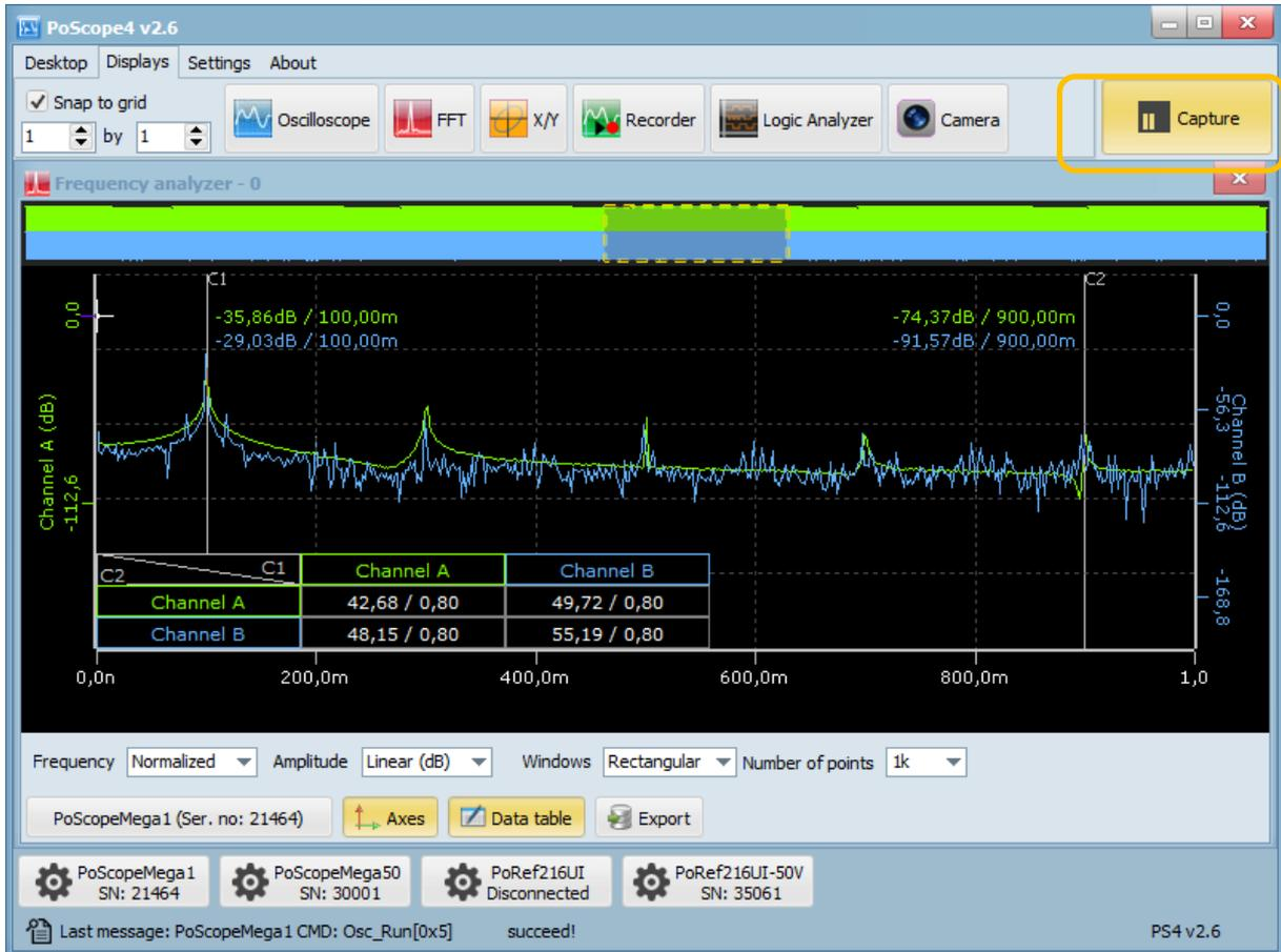
Frequency analyzer in Analyze mode with Overview window
