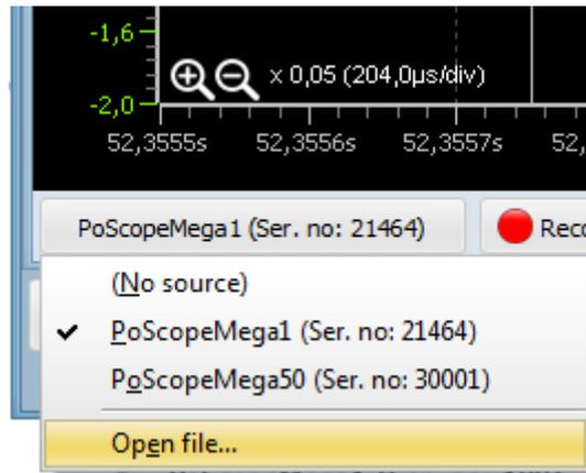
Once open, you can switch pages and resize the overview selector. If you hover over the waveform you can change the timebase using mouse scroller and drag the waveform left and right using you left mouse button. Data table and export features are also available as in the oscilloscope display.
