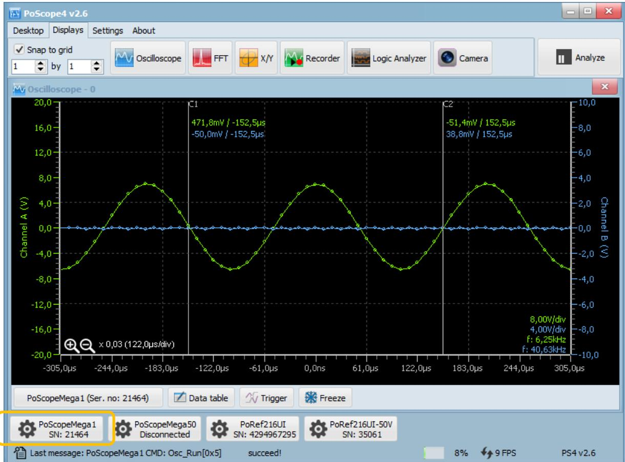
There are two ways how to change voltage range of input. First way to change it by simply left-click & drag channel knob on control GUI or using mouse scroll wheel with mouse positioned above the knob. The second way is to move mouse over the axis on chart and scroll mouse wheel. The result will be same for both methods. Under the settings menu you can invert mouse scroll function if you prefer different behavior when scrolling up or down.
