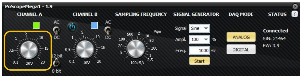
Since the analog generator outputs a voltage amplitude of no more than 2V, you can set the channel A knob to 2V. You will get graphical representation shown below.
