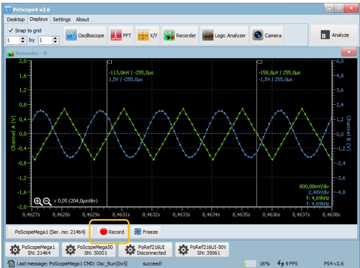
**REMARK:** Record button is visible only if source device is in **PIPE MODE**. Recording is not possible in **BUFFER MODE**.
