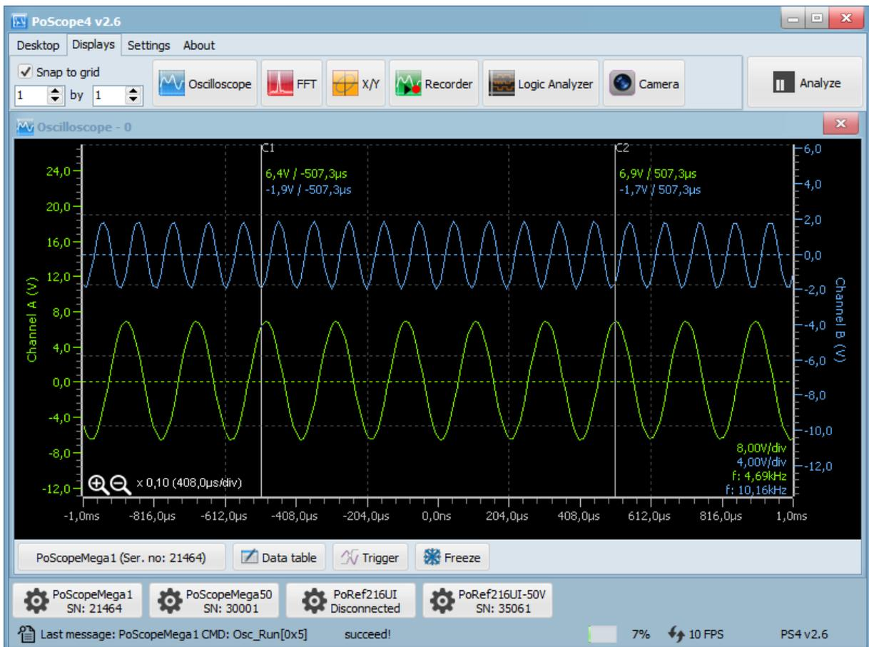
Every device / hardware supported in PoScope4 has dedicated control GUI within PoScope4 environment which is used for control and configuration purposes. Currently supported measurement devices are PoScopeMega1, PoScopeMega1+, PoScopeMega50. Beside measurement devices we offer also generators of voltage/current PoRef216UI and PoRef216U-50V.
