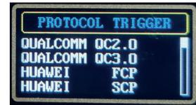
**ATTENTION!** This function increases the output voltage of the USB-C port. Make sure that your connected load is compatible or remove it.
