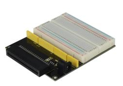
This breakout board makes all contacts of the Micro:Bit easily accessible as a pin socket. In addition, it has a regulated power supply, which makes it possible to operate the breakout board with 5-9V. With the supplied breadboard this breakout board for Micro:Bit is especially well suited to build test or experiment circuits on it. On the freely wireable solder veroboard in the lower half of the board components or whole projects can be soldered for longer use.
