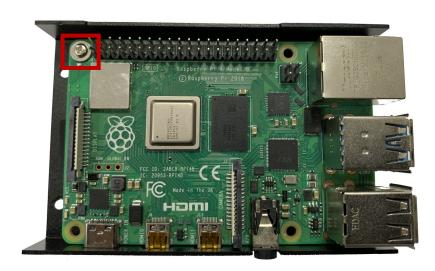
2. Now you can slide the sides into the bottom of the housing and screw them tight.
