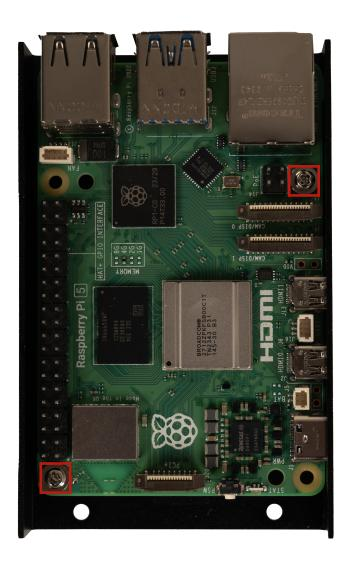
Now attach the enclosed heat sinks to your Raspberry Pi. To do this, remove the adhesive film from the thermal pads and place the heat sinks in the following positions:
