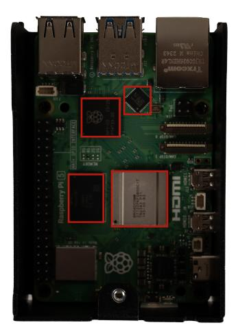
You can now connect the active cooler installed in the housing as standard or simply remove it from the housing. If you want to use the fan, connect the fan cable to the fan connection marked below on your Raspberry Pi 5:
