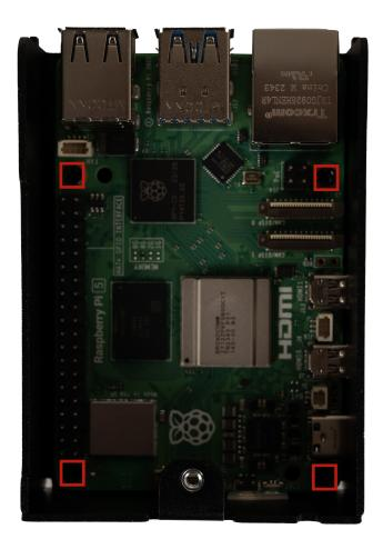
Now attach the enclosed heat sinks to your Raspberry Pi. To do this, remove the adhesive film from the thermal pads and place the heat sinks in the following position:
