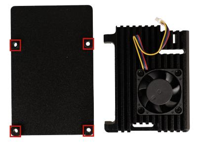
Now attach the supplied thermal pads to the upper part of the housing. To do this, remove the adhesive film from the thermal pads and place the thermal pads in the following positions:
