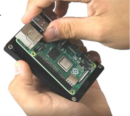
Then the middle (slightly transparent) piece of the case needs to be attached. The magnets will keep it in place.
