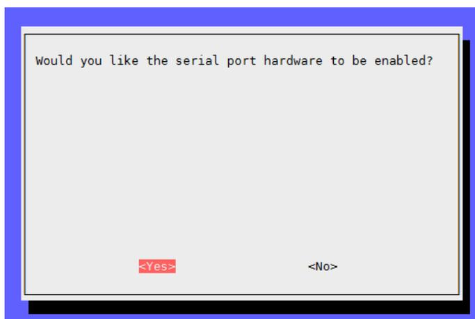
The USB to UART interface of your Raspberry Pi allows you to connect the Pi with your computer and to let them communicate without a connection with the internet.
