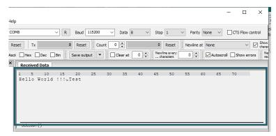
You can open the terminal console via the UART connection instead of an external display or via the internet. Therefore, you can use PuTTY, MobaXterm or others for the connection. For that, you have to change your settings again.
