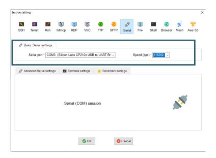
Therefore, you should note that you have to choose the connection type **Serial** and the right port (viewable in device manager) as well as to set the **baudrate** to **115200.**
