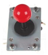
You can also cover the thread with some glue before screwing the head <u>after</u> you mounted it in the acrylic-case. This will fix the head but <u>unmounting the joystick will not be possible anymore.</u>
