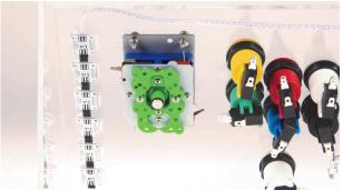
take a nut [F] and screw it tight. Repeat this process with the other three screws.
