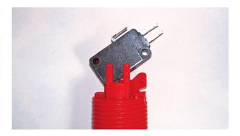
Repeat this step with the other buttons. Make sure that, while placing the buttons, the microswitches don't impede each other.
