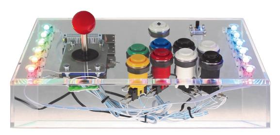
The currently active lightshow is changeable by adjusting the rotary-potentiometer at the topright corner.
