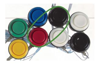
The following menu should appear. You can navigate just like in chapter 3.2 for the command-line setup (Red button: Enter—White Button: Escape).
