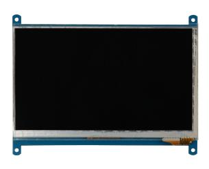
The 7 inch TFT display expands the Raspberry Pi or the Banana Pi with a touchscreen display in no time. It can also be used on any desktop computer and convinces with its high contrast and color-fast display. With a maximum resolution of 1024 x 600 pixels, this display is suitable for any application.
