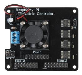
With the help of this expansion board for your Raspberry Pi you can control up to 3 RGB-LED-Matrix rows with the common HUB75 connector, e.g. our Joy-IT RGB-LED-Matrix (LED-Matrix01). In addition, a 25x25mm fan is installed to ensure sufficient cooling of the Raspberry Pi.
