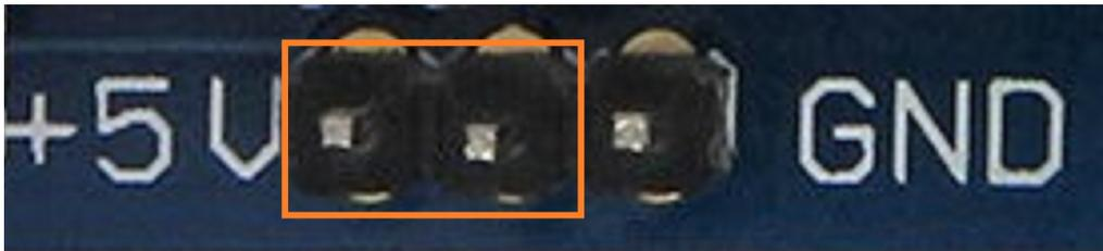
3. However, if you want to supply an external power source, you can install it on the two right pins, marked on the following picture:
