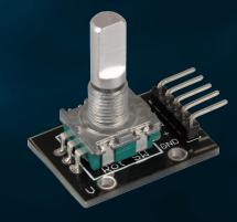
**SUMMARY:** We use the rotary encoder to control the color and brightness of our four LEDs. Turning the encoder changes the brightness, while pressing the encoder adjusts the color of the LEDs.
