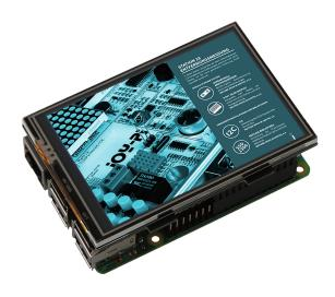
With the 3.5 inch TFT touchscreen display you can build a mini tablet PC based on a Raspberry Pi in no time.
