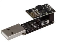
Once you have successfully installed the board, you can select the **Generic ESP8266 Module** from the list of available boards.
