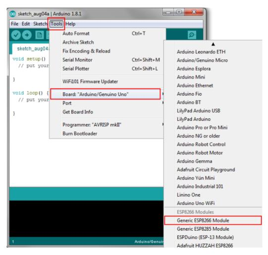
Your Arduino development environment is now prepared for the use with an ESP8266.
