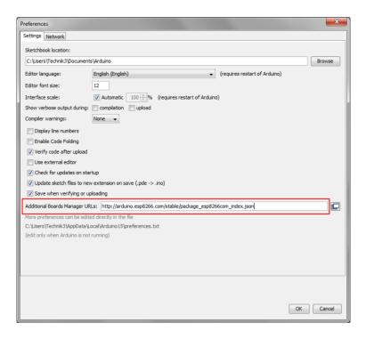
Next, an additional board library must be installed. Open the board manager and install the **ESP8266** library.
