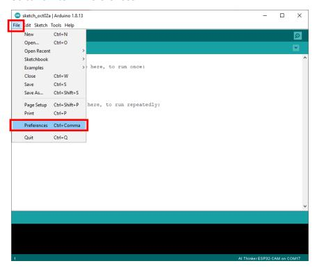
Add the URL: <a href="https://dl.espressif.com/dl/package\_esp32\_index.json">https://dl.espressif.com/dl/package\_esp32\_index.json</a> under Additional Board Manager URLs. Multiple URLs can be separated with a comma.
