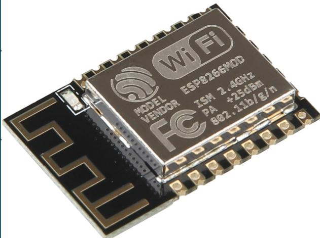
The ESP12-F is an ultra-low power UART WiFi module specifically designed for the needs of the networked world. It offers an outstanding range of functions in a small package. Specially developed for mobile devices and the Internet of Things, the ESP12-F provides a stand-alone network solution.
