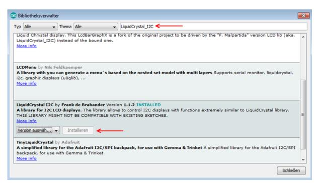
As soon as the library is installed, the installation of the display is finished. You can now transfer the code example which is described in the next step and test the display
