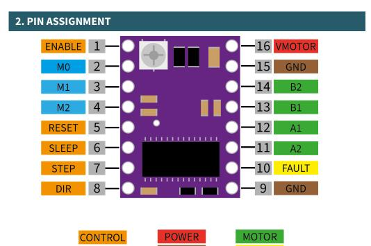
• **ENABLE**: This pin is used to disable the driver when this pin is set to high (H) and to enable it when set to low (L). Internal pull-down resistor is present.
