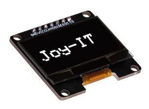
This graphical 1.3" OLED display has a resolution of 128 x 64 pixels and communicates via the SPI interface. Optionally, the display can also be soldered to the I2C interface on the back. This makes the display particularly universally applicable.
