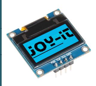
This small 0.96 inch (approx. 2.44 cm) OLED display with SSD1306 controller works with an I2C interface, making it easy to use with Arduino, Raspberry Pi or other single-board computers or microcontrollers.
