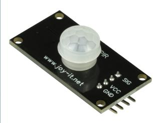
The sensor on this module is a pyroelectric infrared sensor which detects movement in the detection area of the Fresnel lens and then outputs a "HIGH" signal at the sensor output pin "SIG" for 3 seconds. Afterwards the signal changes back to the "LOW" state. The soldered potentiometer is used for continuous range adjustment. With the help of this module and a microcontroller such as Raspberry Pi or Arduino, it can be used for safety systems or automation, among others.
