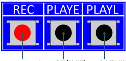
**REC:** Is Active-HIGH and has priority over the P-E and P-L signals. When the pin is set to HIGH, this activates the recording. The recording runs as long as the pin is set HIGH. Not longer than the set recording time.
