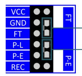
FT Jumper (Feed Through): Allows the microphone to output directly to the speaker.
