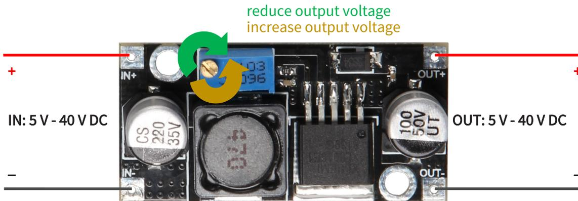
Connect the voltage converter with the contact IN+ to the positive pole and with the contact IN- to the negative pole of your DC voltage source.
