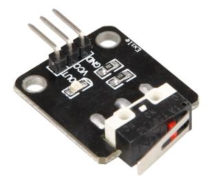
Our bump sensor automatically detects contact with an obstacle and sends the digital signal to a corresponding device via the output pin.
