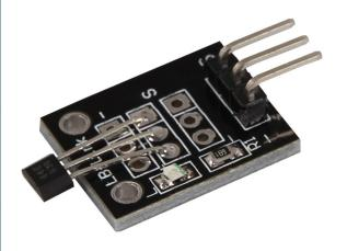
With this small Hall magnetic field sensor, you can detect magnetic fields using the sensor's digital output and the integrated status LED. When the sensor is held in a magnetic field, the LED lights up and the sensor output switches to low state.
