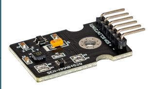
This digital, intelligent and capacitive MEMS- acceleration sensor is powerful and an absolute all-rounder regarding output, voltage supply and interface voltage. The MMA8352Q offers freely selectable measurement ranges up to 8g with high-pass filtered Data as well as unfiltered data in real-time.
