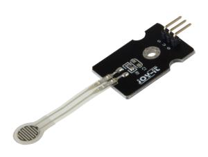
This pressure sensor works using analog resistance detection, when an external pressure is applied to the sensor, the resistance and thus the voltage of the analog signal changes. The sensor is highly sensitive, and the sensor strip is water-proof and flexible.
