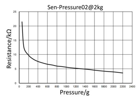
The diagram shows the pressure-resistance relationship for the entire resistance range.
