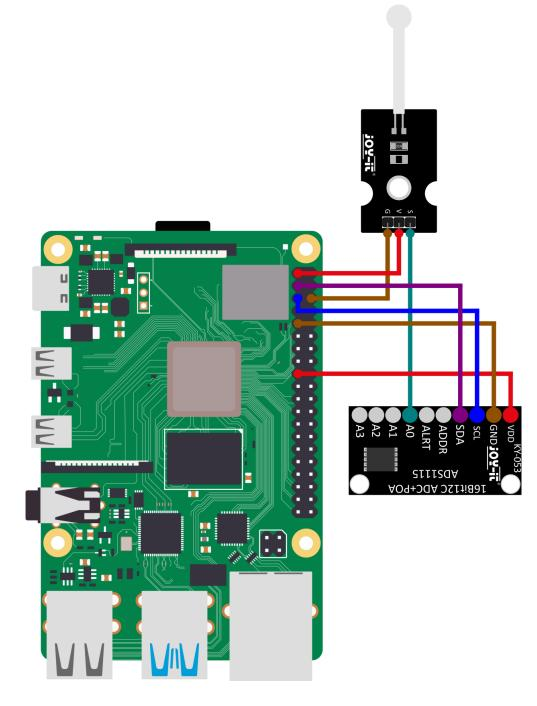
We provide a code example for use with the Raspberry Pi which you can download <u>here</u>. To be able to use the ADC you have to activate I2C first.
