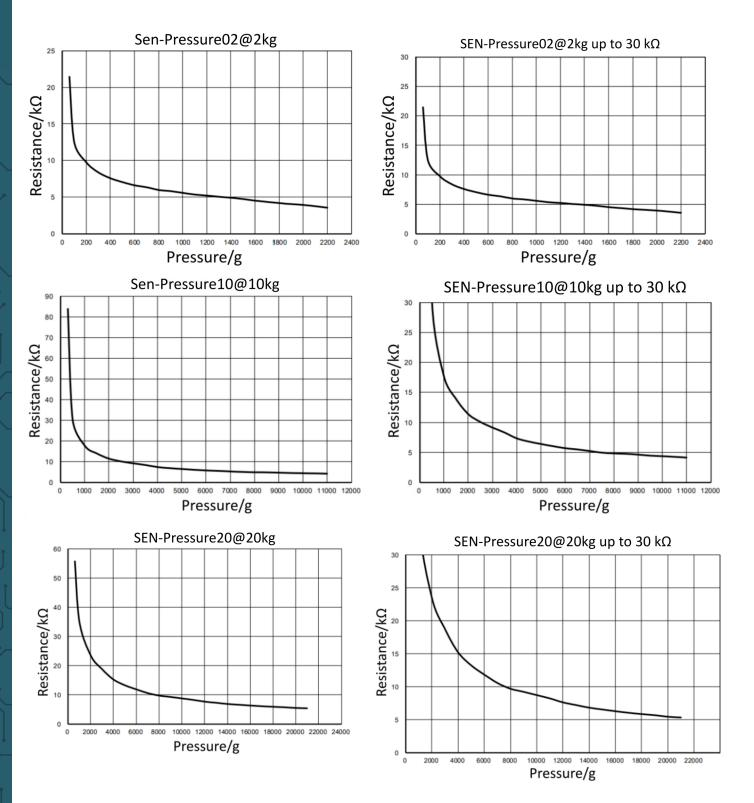
The diagram on the left shows the pressure-resistance relationship for the entire resistance range.
