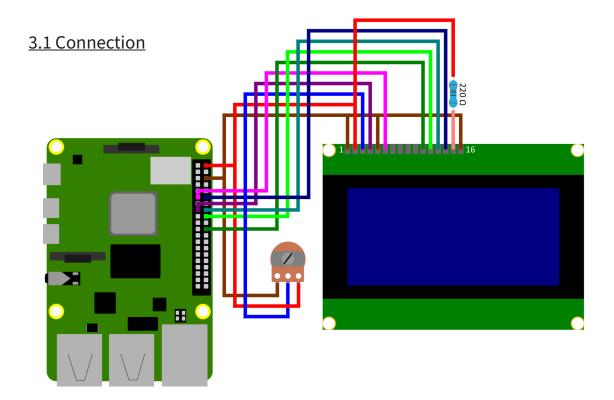
Since the display works with a 5V logic level, you must use a logic level converter if you want to read data from the display with the Raspberry Pi. In this example, the display is only written to, so the Raspberry Pi can be connected directly to the display.
