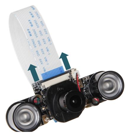
Next, you can now simply remove the ribbon cable and insert the appropriate ribbon cable for the Raspberry Pi 5 and **push the clip in the opposite direction of the arrows shown above to reattach the ribbon cable.**
