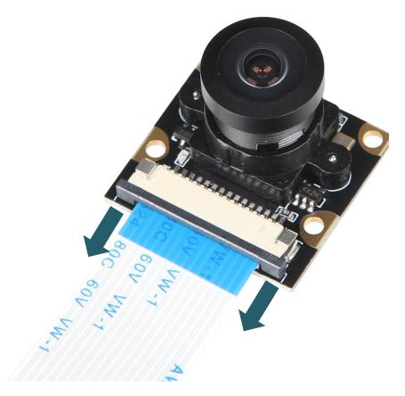
Next, you can now simply remove the ribbon cable and insert the appropriate ribbon cable for the Raspberry Pi 5 and **push the clip in the opposite direction of the arrows shown above to reattach the ribbon cable.**
