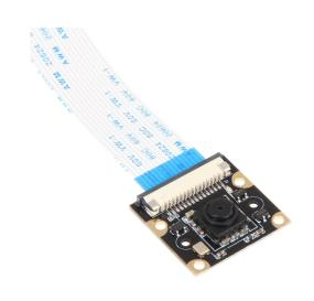
This camera module is for all Raspberry models and works with the familiar OV5647 chip. It provides good images with 5MP quality.
